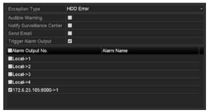
Figure 12-29 Configure HDD Error Alarm
