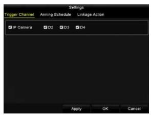
Figure 5-18 Set Trigger Camera of VCA Alarm
