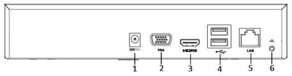
Figure 1-8 HWN-2100MH Series Rear Panel
