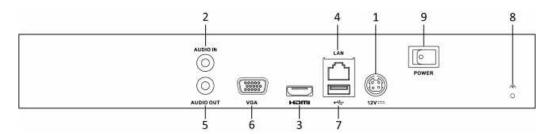
Figure 1-14 HWN-4100MH and HWN-4200MH Series Rear Panel
