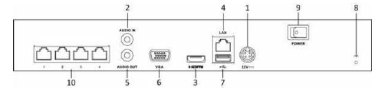
Figure 1-15 HWN-4100MH-P Series Rear Panel
