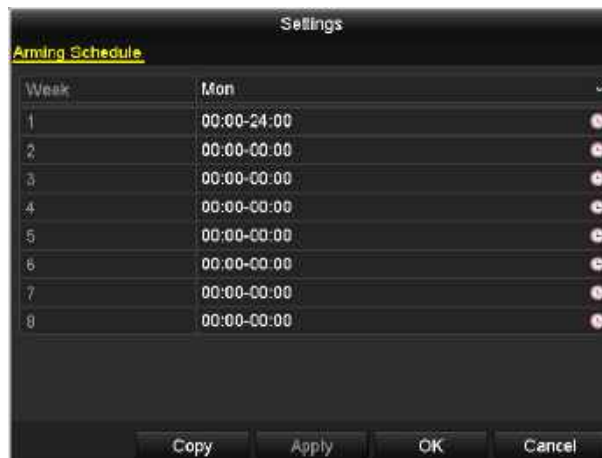
Figure 8-17 Set Arming Schedule of Alarm Output
