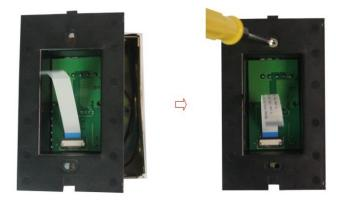
4. Cover touch panel Look at the direction of touch panel, install the ribbon cable, and then cover the touch panel.
