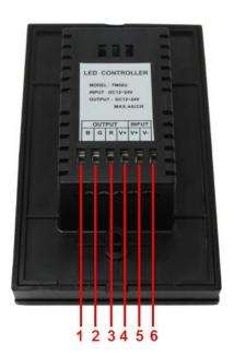
5 and 6: power input, input voltage range: 12-24V, 5 for positive, 6 for negative. 1,2,3 and 4: power output, output voltage is 12-24V, Max output current is 8A, 4 for positive, 3 for red led interface, 2 for green led interface, 1 for blue led interface.
