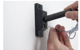
Step 10 Plug the led strip connector into the female base connector, Take out the screw and fix it on the drilled wall. Repeat the operation on the other end.
