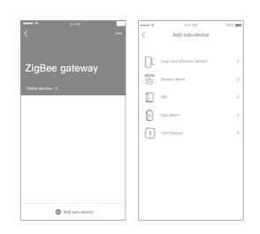
Press and hold the reset button for 5 seconds, until the network indicator light begins flashing. Follow the App instructions to add the device.
